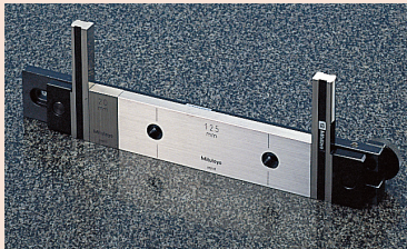
Use of B-type connectors in gauge construction
