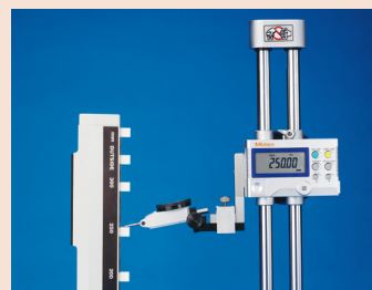
Checking accuracy of height gage
