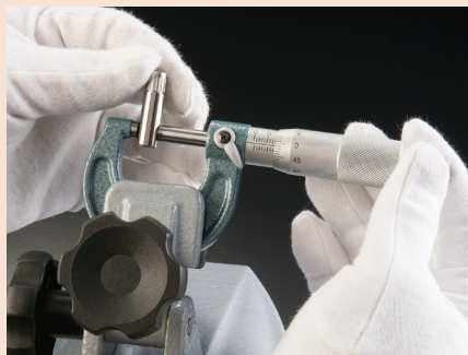
Metric Micrometer set / With ratchet thimble
