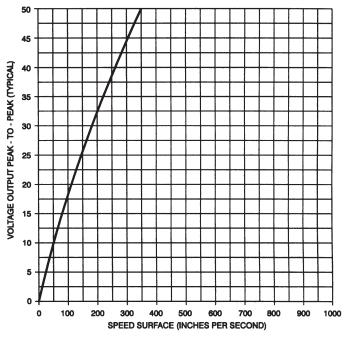
Shows peak-to-peak voltage output vs. surface speed of a 20-pitch, 30 tooth ferromagnetic gear at 0.005 inch clearance. Load = 100,000 ohms.
