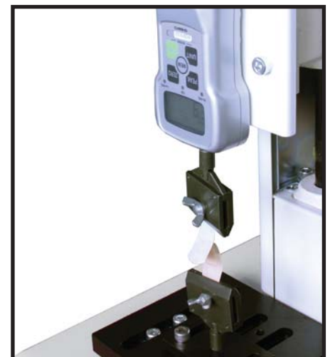
Stand with Optional Grip Performing Peel Test
