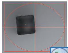
Area Centroid Tool This tool detects the position of a form's centroid, and is suited to the positioning of different forms.
